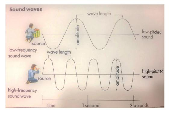
Figure 5.2: "Measuring Sound Waves"<sup>346</sup>
